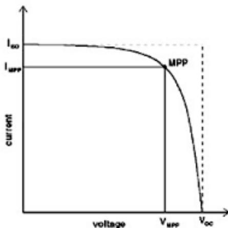
**Figure 1:** Solar cell characteristic curve
